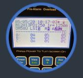
In addition, the large 21 character x 8 row backlit LCD display can show all four phase currents with their percentage of Ir, and when in overload, the Thermal Content % - as well as date & time, battery status, the ACB's main characteristics, Long Time (LT) Ir value, the Trip Unit "modelled", and all the protective functions and options' ON / OFF status'.
